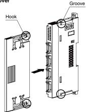
The protective cover is to be attached over the connected I/O module at the right end.
