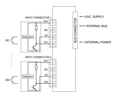
Note: For dry contact input, connect it across the terminals 3 and 4.
