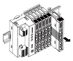
• Removing an intermediate module
