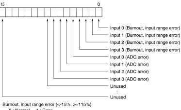
0 : Normal 1 : Error ADC error (no response from ADC) 0 : Normal 1 : Error
