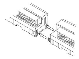
3) Mount the combined module on a DIN rail.
