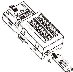
B) Set the upper hook at the rear side of the unit on the DIN rail.
