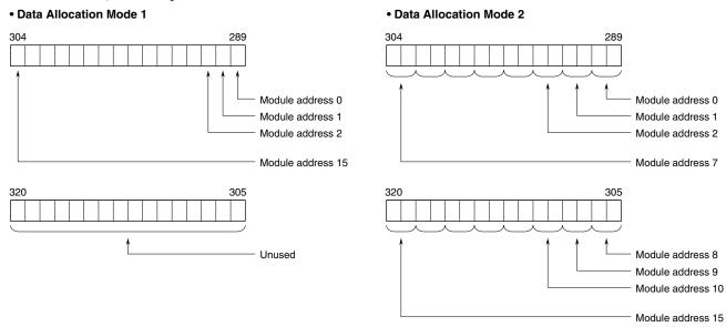
In the Data Allocation Mode 2, the LSB is used for channel 1, and the MSB for channel 2, of an analog module.
