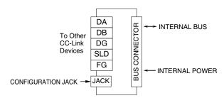
Note: The FG terminal is not connected with the FG of the power supply module (Model: R6x-PF1 or R6-PSM).
