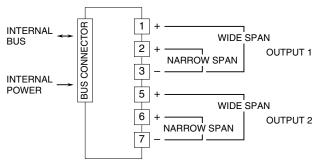
• Wide span: -10 – +10 V DC, -5 – +5 V DC, 0 – 10 V DC, 0-5~V~DC,~1-5~V~DC
