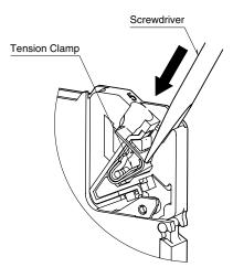
Insert a wire. Push the screwdriver toward the direction indicated with the arrow in the figure below to widen the opening if necessary.
