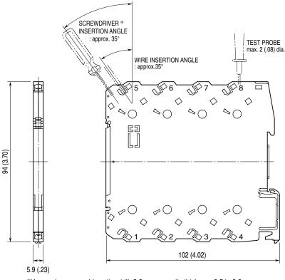
\*Use a minus screwdriver: tip width 3.8 mm max., tip thickness 0.5 to 0.6 mm
