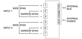
Wide span: -40 - +40 mA DC, -20 - +20 mA DC, 0 - 40 mA DC, 0 - 20 mA DC, 4 - 20 mA DC
