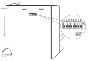
Counter Reset SW is normally OFF during operation.
