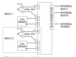
\*For dual redundant communication. Note: The section enclosed by broken line is with 2-ch. option.
