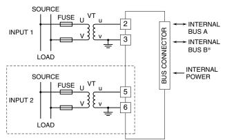
\*For dual redundant communication. Note: The section enclosed by broken line is with 2-ch. option.
