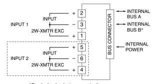
\*For dual redundant communication. Note: The section enclosed by broken line is with 2-ch. option.
