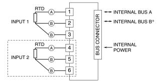
\*For dual redundant communication. Note: The section enclosed by broken line is with 2-ch. option.
