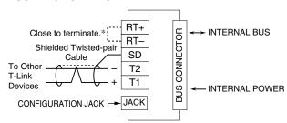
\* When the module is at an end of the transmission line via twisted-pair calbe (= when there is no cross wiring), close across the RT+ and RT-terminals with the jumper included in the product package. Remove the jumper for all other locations.
