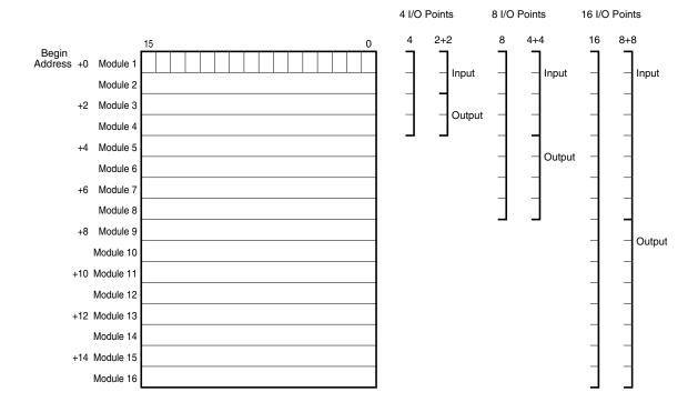
Total number of modules equal the assigned I/O points with Data Allocation Mode 1. I/O modules can be allocated from I/O Module Slot No. 1.
