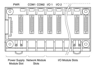
The Network Interface Module must be mounted on the COM1/COM2 on the Base.
