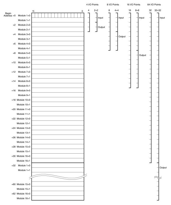
Total number of I/O modules are half the assigned I/O points with Data Allocation Mode 2. I/O modules can be allocated from I/O Module Slot No. 1.
