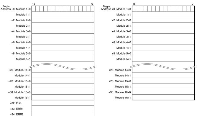
The area enclosed with a bold line is assigned for I/O data.
