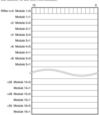
Each module takes two-word areas for input and output respectively, regardless of whether the module type is input or output. If a module for Data Allocation Mode 1 is used, all the bits for Module n+1 data turn to "0" (unused).
