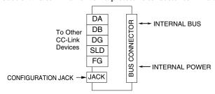
Note: The FG terminal is not connected with the FG of the power supply module (model: R5-PS).
