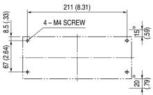
\*Working space required for mounting/unmounting the modules.
