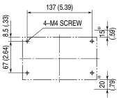
\*Working space required for mounting/unmounting the modules.
