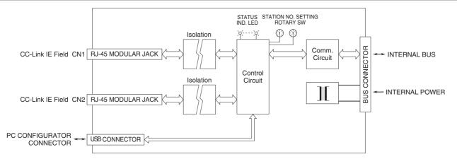
Regarding CN1 and CN2 of RJ-45 connector for CC-Link IE Field network, there is no restriction for connection order.
