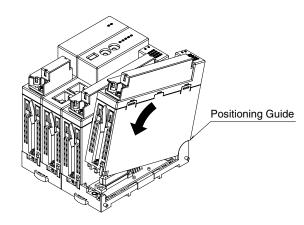
3) Tighten the base fixing screw using a screwdriver (stem length: 70 mm/2.76" or more) (torque  $0.5 \text{ N} \cdot \text{m}$ ).
