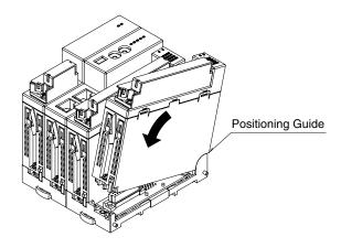
3) Tighten the base fixing screw using a screwdriver (stem length: 70 mm/2.76" or more) (torque 0.5 N·m).
