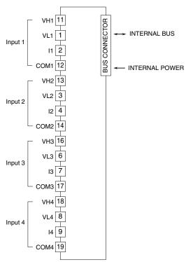
Note: Connect either wide or narrow span or current terminals for each channel.
