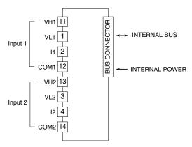
Note: Connect either wide or narrow span or current terminals for each channel.
