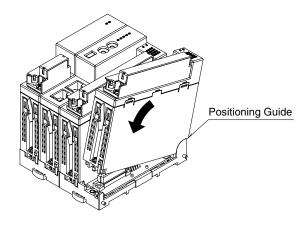
Tighten the base fixing screw using a screwdriver (stem length: 70 mm/2.76" or more) (torque 0.5  $N \cdot m$ ).
