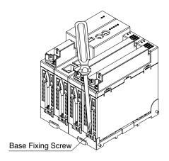
While pressing the projection on the lock tab, push the module upward.
