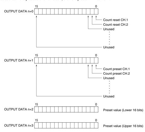
Note: When reset and preset are simultaneously output, reset overrides preset.
