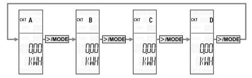
Measurable circuits are different depending on the system configuration. For unmeasurable circuits, switch by  $\boxed{MODE}$  button is skipped.
