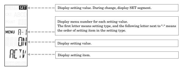
Press the following buttons to switch setting value display or change the setting value.
