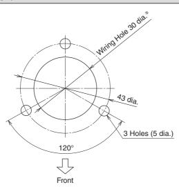
\* Protect wires to prevent scratching them at the edge of the compartment.
