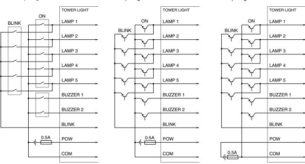
Note 1: Do not set lamp ON input to "On" and BLINK input to "Blink" at the same time watsoever, it might result in shortcircuit.
