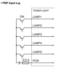
Note 1: NPN input and PNP input are available only for 24 V DC.
