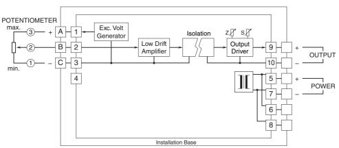
Note: Use shielded cables for I/O wiring.
