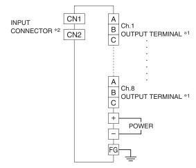
\*1 Terminal A: positive output, Terminal B: negative output \*2 CN2 is not provided for M80BS-821
