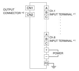
\*1 Terminal A: positive input, Terminal B: negative input \*2 CN2 is not provided for M80BS-811 Note: Use shielded cables for I/O wiring.
