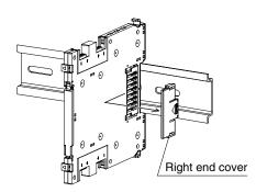
2) Remove the left end cover of the unit to be mounted next, pull out the upper and lower sliders, and slide the upper and lower tabs to the left.
