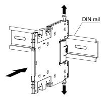
3) Push the sliders back into the body to fix the unit to the DIN rail.
