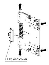
3)Attach the unit to be mounted onto the DIN rail while sliding its male power connector along the female power connector of the already mounted unit so as to engage with each other. Confirm that the upper and lower tabs fit into the respective concave portions of the already mounted unit.
