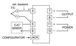
\* The CJC Sensor is secured to the terminal 6. Loosen only the terminal 4 – 5 and connect the T/C extension wires.
