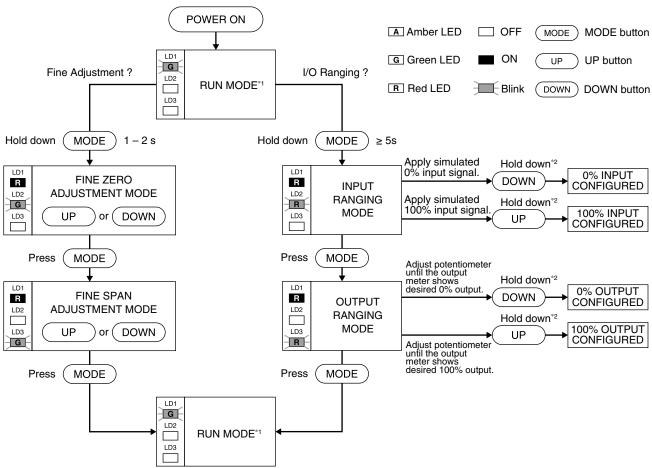
\*1 In the RUN Mode, the green LD1 blinks (PC configuration), or turns on (DIP SW configuration).
