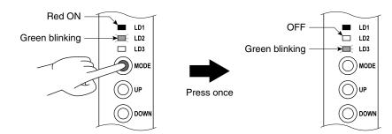
• Press MODE button once to go on to the Fine Span Adjustment Mode.
