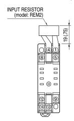
Input shunt resistor attached for current input.
