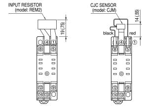
Use the input resistor (model: REM2) for a DC current input, and the CJC sensor (model: CJM) for a thermocouple input, both included in the package.
