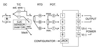
\*Input shunt resistor attached for current input.
