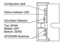
The front cover cannot be opened to 180 deg. when flush with neighboring units.
