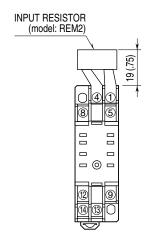
Input shunt resistor attached for current input.
