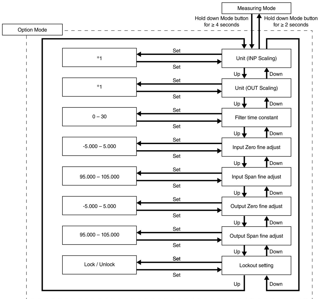
\*1. Refer to [60] Unit (INP Scaling) or [61] Unit (OUT Scaling) for usable unit.
