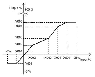
When the input to be converted does not match any X value in the table, two X values which are closest to the input in positive and negative directions are selected and linearly interpolated, thereby obtaining a Y value to be outputted.
