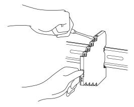
Hold the module steady at the front when you tighten/loosen screw terminals.
