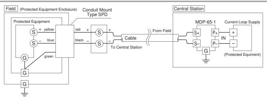
Connect the Conduit Mount Type SPD's green leadwire to the ground terminal inside the protected equipment enclosure to ground through the enclosure's outside ground terminal.
