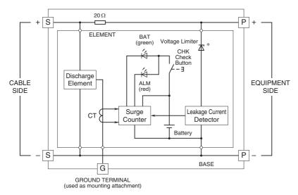
\* The zenor diode has polarity. Zero-cross signal cannot be connected.
