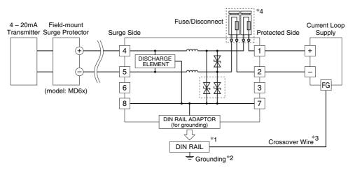
\*1. Oxide film on the surface of an aluminium rail may lower the electric conductivity between this module and the ground. Use a steel or copper rail.
