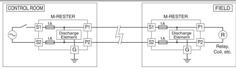
The M-RESTER must be connected with its terminals S1 and S2 faced on power source side in order that the fuses would be blown in case of shortcircuit of the discharge element.
