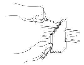
Hold the module steady at the front when you tighten/loosen screw terminals.
