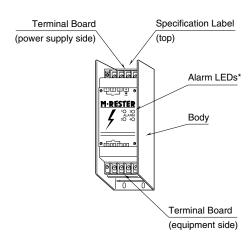
\*Two LEDs for two-wire power line
