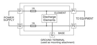
Note: When the head element is removed, the line will be open.
