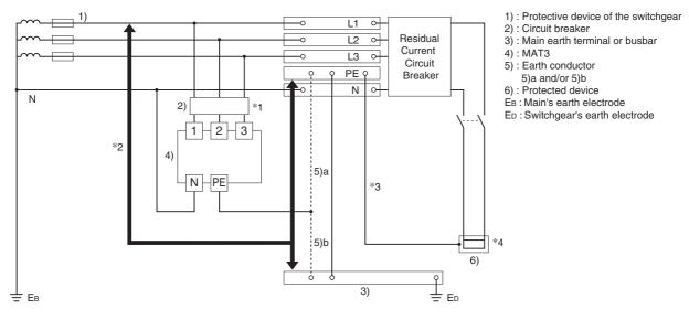
\*1. The circuit breaker or the fuse as disconnectors must be installed.
