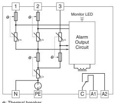
6: Thermal breaker Note: Terminals C, A1 & A2 are available for 'Alarm output' code 'A.' The schematic shows the relay contact status of a thermal trip or power off.
