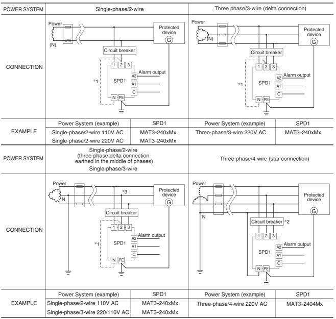
\*1. For TT system, in order to ensure safe failure mode at TOV due to earth fault on high-voltage systems, connect between terminal 2 and N of the MAT3. \*2. For TT system, in order to ensure safe failure mode at TOV due to earth fault on high-voltage systems, install a four-pole (three-pole plus neutral) circuit breaker.
