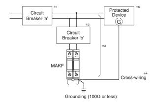
\*1. The circuit breaker must be installed.
